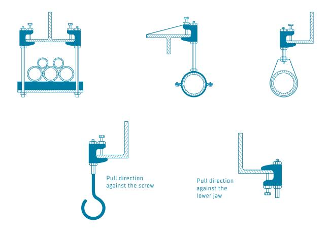
Our type TK and TKN beam clamps can be fixed with the pull direction against the set screw or against the lower jaw. Please see our installation instructions for further information.
