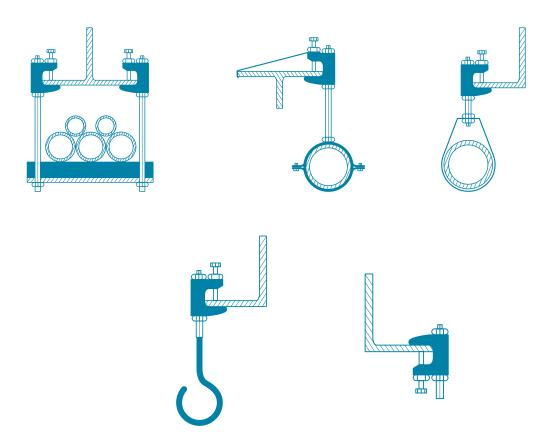
Our type TK and TKN beam clamps can be mounted with the tensile direction against the retaining screw or against the support. Please see our mounting instructions for further information.
